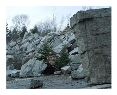
Abandoned at the foot of a jumbled pile of granite lies the old pole head with remnants of wire ropes still attached. Once affixed at the top of a rotating mast, the pole head, derrick, and boom system could lift and manipulate the weighty blocks of granite.
